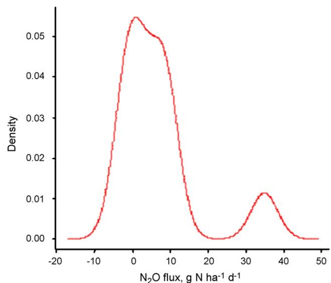
**Fig. 1.** Distribution of data set collected from 10 chambers in Rowden, 20/4/6 in the 0N paddock. Values were: 6.9, 9.8, 2.0, 34.8, 9.2,  $-2.8$ , 0.19, 0.90,  $-1.68$ ,  $6.8 \text{ g N}_2\text{O ha}^{-1} \text{ d}^{-1}$ . The normal mean was 6.6, the 2 group mean was  $14.2 \text{ g N}_2\text{O ha}^{-1} \text{ d}^{-1}$ .
